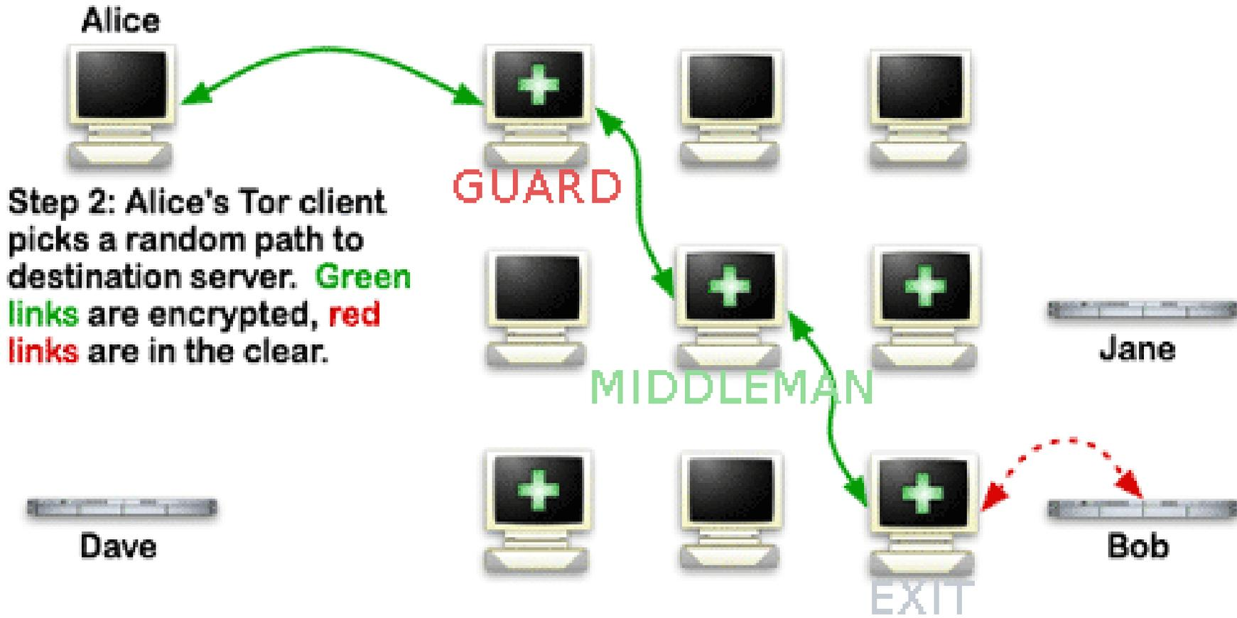
Step 2: Alice's Tor client picks a random path to destination server. Green links are encrypted, red links are in the clear.
